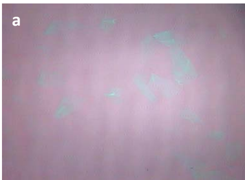
Optical microscope images 561x467μm: a) GO on SiO 300nm, b) thermally reduced GO on SiO 300nm
